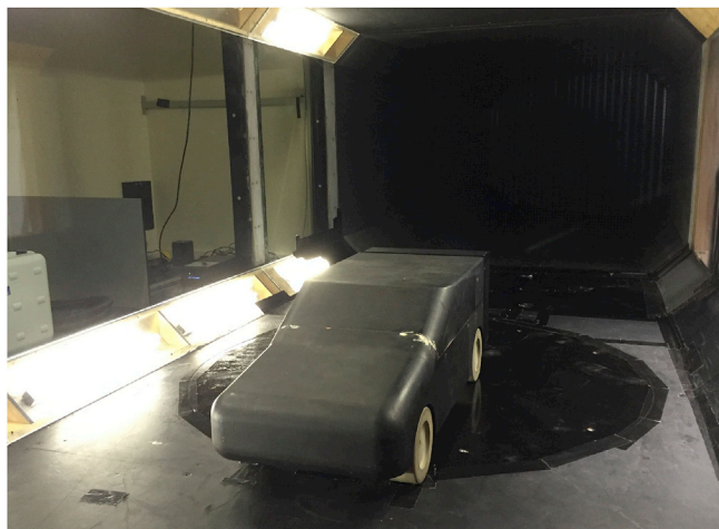
Fig. 2. Generic SUV inside the test section of the wind tunnel at Loughborough University.
