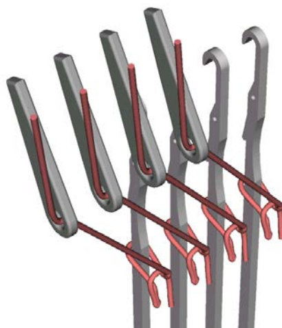
Figure 1. Needle Rise After a Two-Needle Underlap
