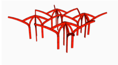
Option 1A Concrete main arch members tied back to a central 9m x 9m arch
