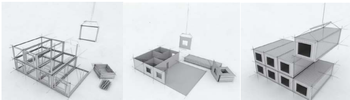
Figure 2.1 a) Elemental sub-assembly, b) planar and c) volumetric building methods (source: Buro Happold)
