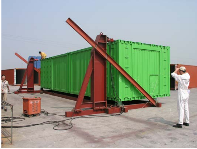
Figure 2.4 Load testing of prototype container (source: Verbus)
