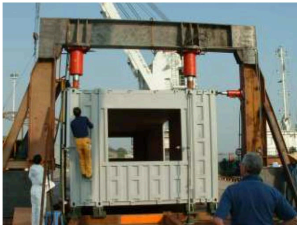
Figure 4.43 Load testing of the multi-storey unit prototype
