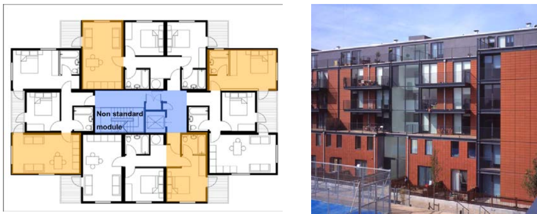
Figure 4.16 Social Housing layout of standard 3.6 m wide modules based on Lillie Road
