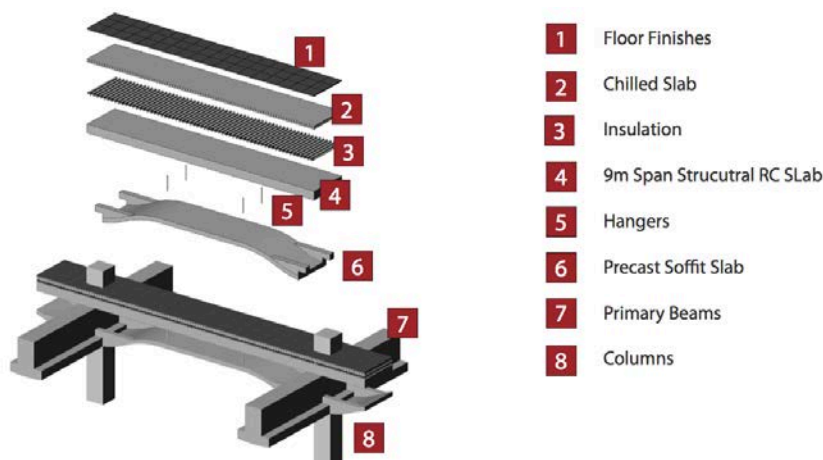
Figure 5.11 Concourse element arrangement (source: Buro Happold).
