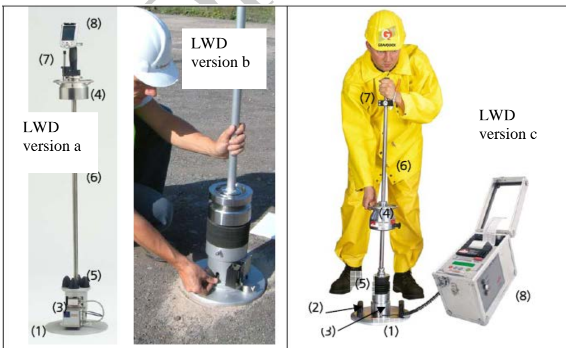
Figure 1. Three types of light weight devices commonly used in Europe.
