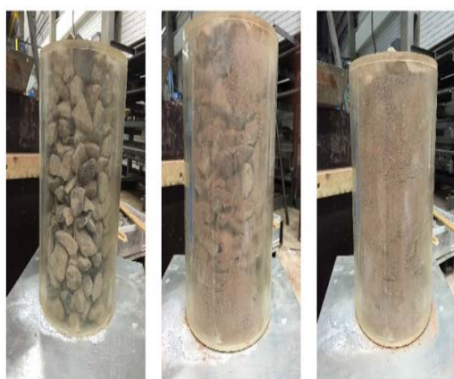
Figure 3 Representation of 3 fouling states using R_{FV} = 100\% , R_{FV} = 50\% and R_{FV} = 0\% :
