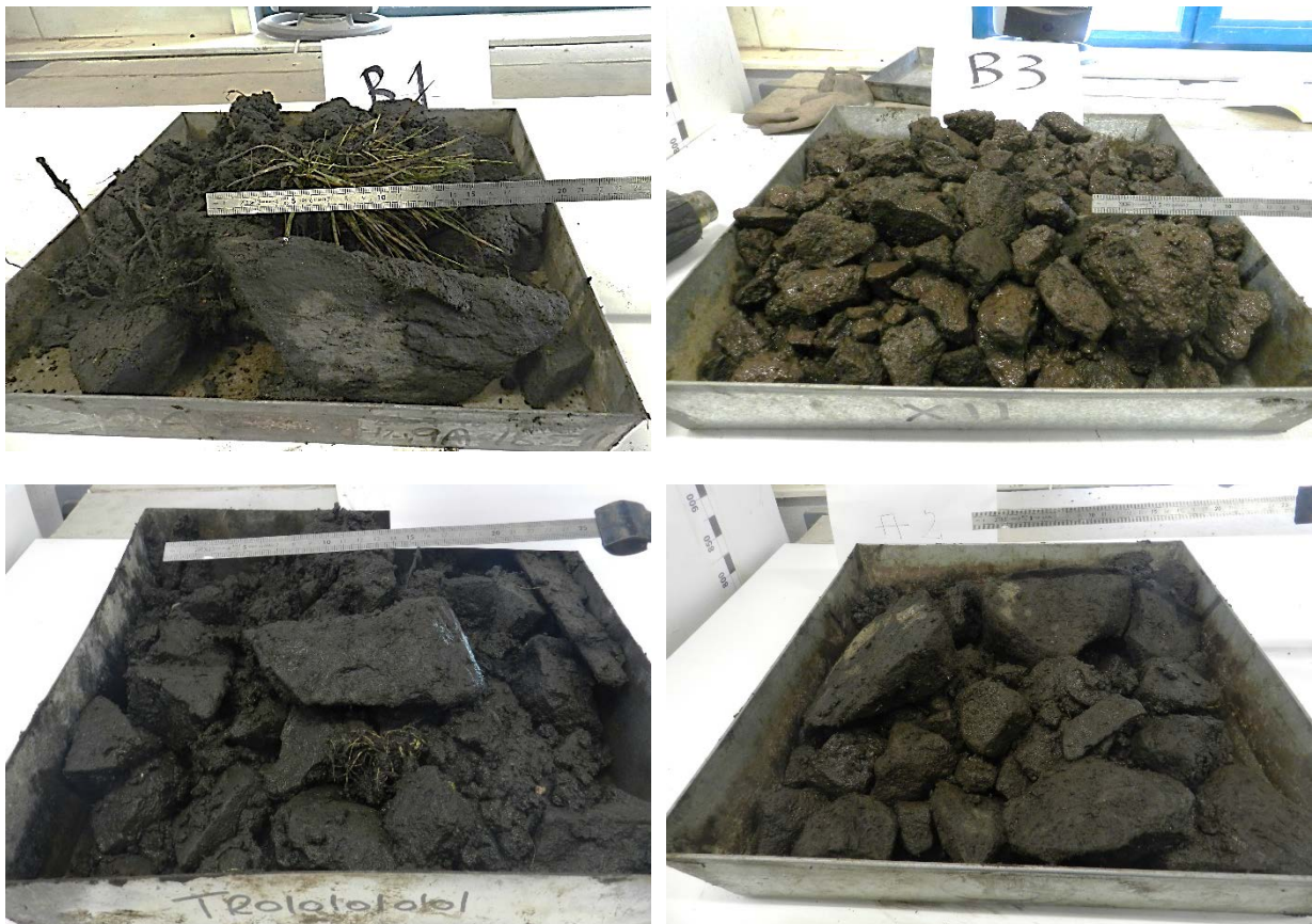
Figure 19 Samples from M77/GSO sieving exercise; oversized aggregate can be observed in B1 sample (top up) moderately fouled Type B material on B3
