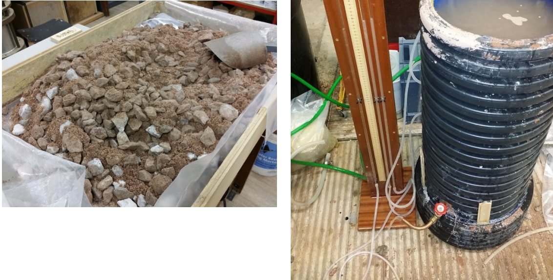
Figure 24 Material Mixing at the lab and Permeameter used in trials
