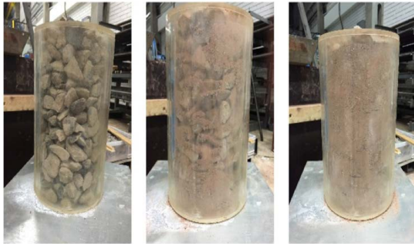
Figure 21 Effect of increasing R_{FV} ; from left to right: R_{FV} = 1 R_{FV} = 0.5 and R_{FV} = 0
