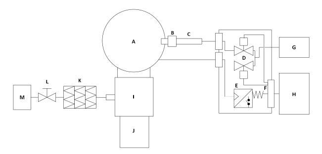
Figure 2.2.4. Schematic diagram of adaptive breath sampling system. (A) full face breathing mask; (B) PTFE connector with sampling capillary; (C) adsorbent tube; (D) micro-control valves; (E) pressure transducer; (F) electronics interface; (G) sampling pump; (H) Laptop computer running DAC card and Labview software; (I) PTFE T-piece connector; (J) one-way valve; (K) 3-stage filtration assembly; (L) pressure regulator; (M) air supply generator.
