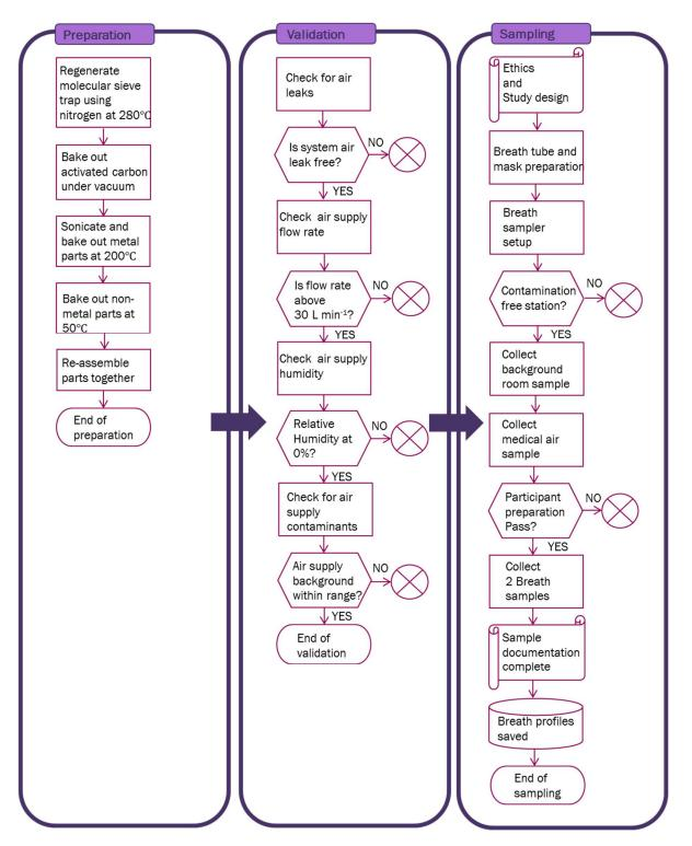
Figure 4.4.1.1. Work-flow chart detailing the exhaled breath analysis method using the portable adaptive breath sampler including preparation, validation and sampling stages
