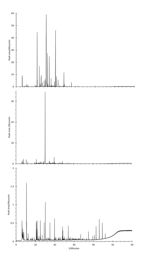
Figure 3.4.1.1. TIC chromatogram of storage sample set including participant breath sample (top), medical air supply sample (middle) and background room air sample (bottom).
