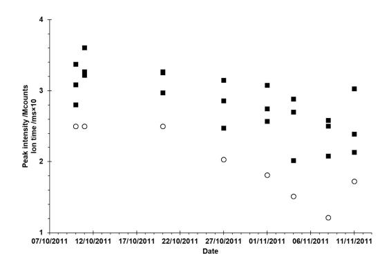
Figure 3.2.3.2.2. Peak areas of toluene-d<sub>8</sub> internal standard measured from 22 breath samples (black squares) and ion time measured before sample analysis (white circles) plotted against analysis date for one month duration.
