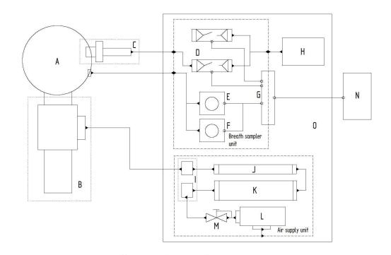
Figure 4.3.1.1. Schematic diagram of portable adaptive breath sampler illustrating the main components: breath mask (A), mask air supply assembly (B), adsorbent sampling assembly (C), micro-control valves (D), pressure transducer (E, F), electronic interface (G), precision air sampling pump (H), dust filter (I), activated charcoal filter (J), molecular sieve 13X filter (K), air supply pump (L), pressure regulator (M), laptop containing DAC card and labview software (N) and portable suitcase (O)
