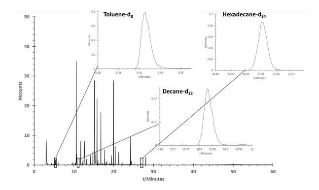
Figure 3.2.3.1. TIC chromatogram of 2.5 L breath sample doped with internal standards toluene- $d_8$ , decane- $d_{22}$  and hexadecane- $d_{34}$ . The EIC chromatogram of the three internal standards are shown on the right hand.
