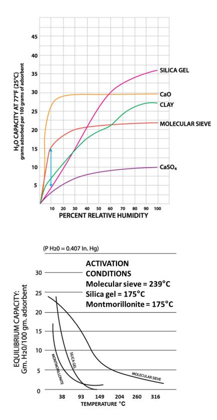
Figure 4.2.3.2.2. (top) Desiccant water capacity versus relative humidity based on air at atmospheric pressure and 25°C. (bottom) Desiccant water capacity versus temperature (77).
