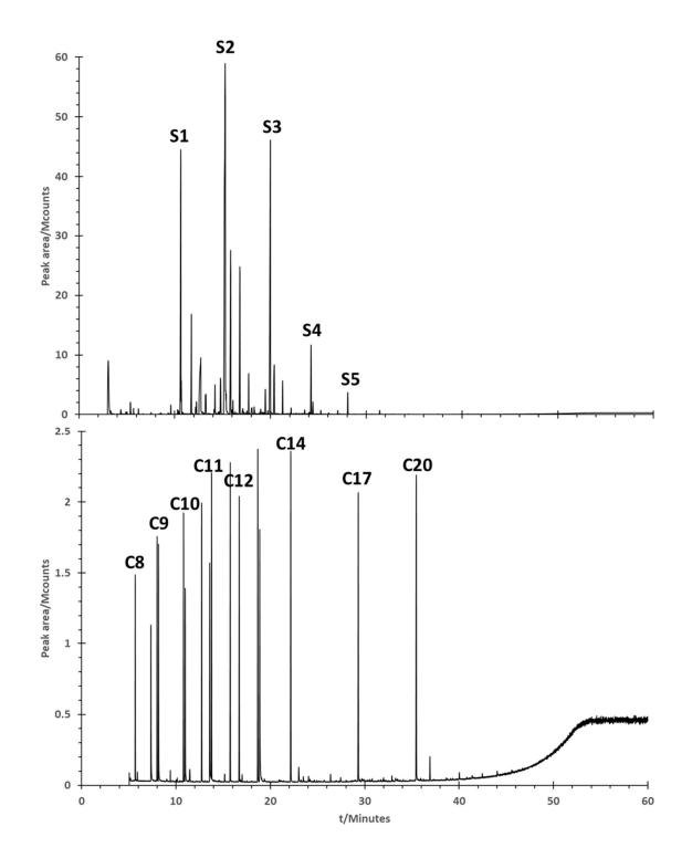
Figure 2.4.3. TIC chromatograms of primary retention index ladder using alkane compounds from C8 to C20 (bottom) and secondary retention ladder using breath cyclosilane compounds from S1 to S5 (see Table 2.4.3.2.) (top)
