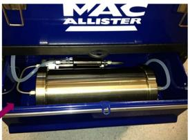
Air supply unit Containing high flow air pump
