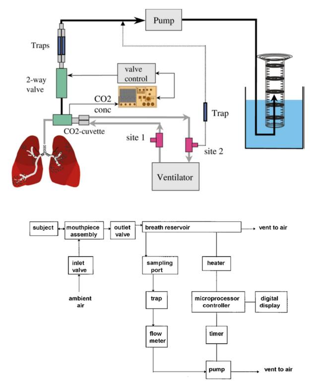
Figure 1.6.2. Sampling devices which collected alveolar air. (Top)  $CO_2$  controlled sampling of alveolar gas in mechanically ventilated patients by Schuert *et al* (48) (Bottom) Breath collecting apparatus (BCA) developed by Philips *et al* (49).
