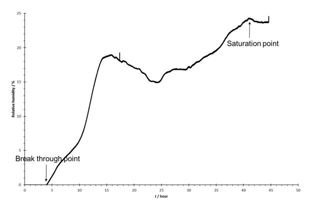
Figure 4.5.1. Line plot of RH% against dehydration duration using molecular sieve 13X desiccant filter. Both break through point and saturation point are labelled on the graph
