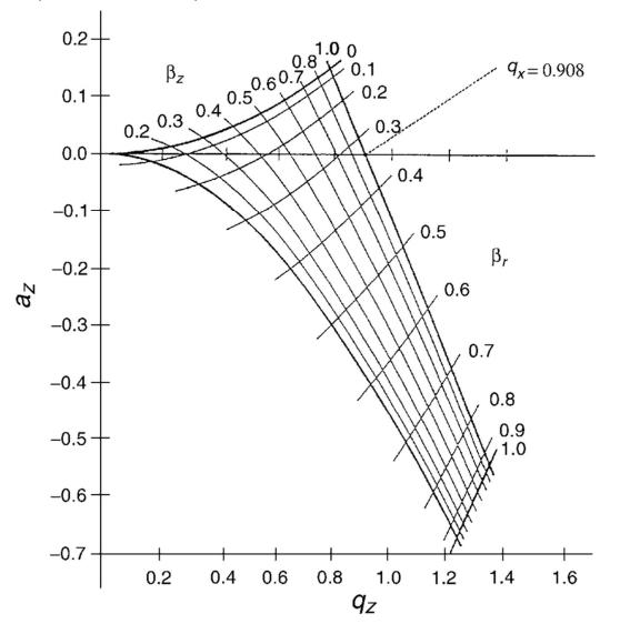
Figure 1.6.4.3.2. The Mathieu stability diagram for quadruple ion trap (58). Ion are simultaneous stable in both the R- and Z- planes if their  $a_z$  and  $q_z$  are within the
