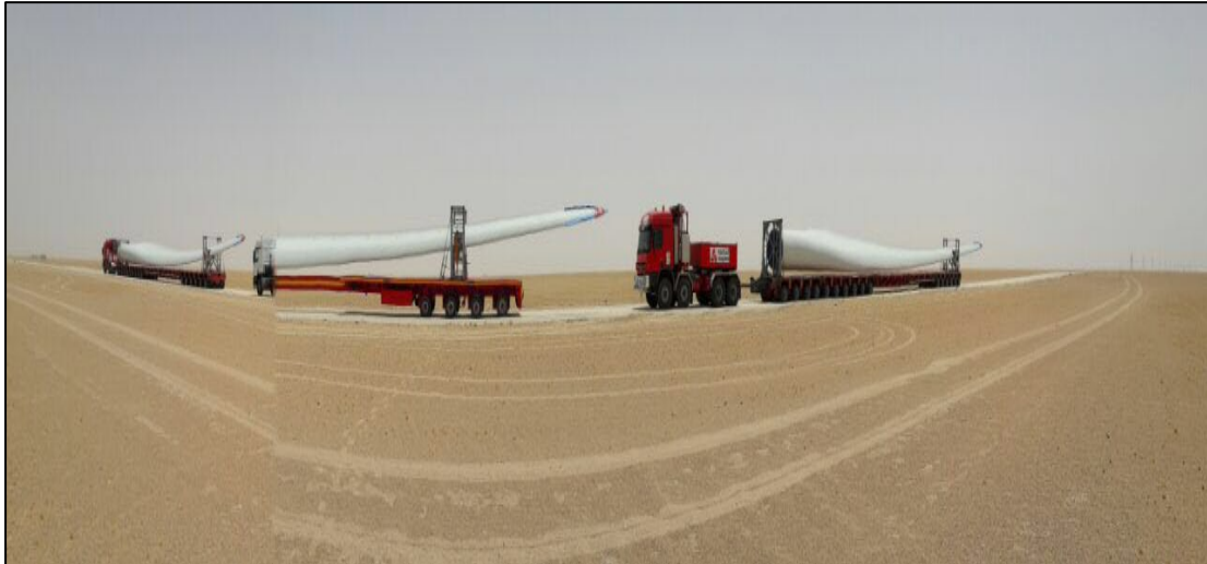
Figure 5.4 Trailers used to transport blades
