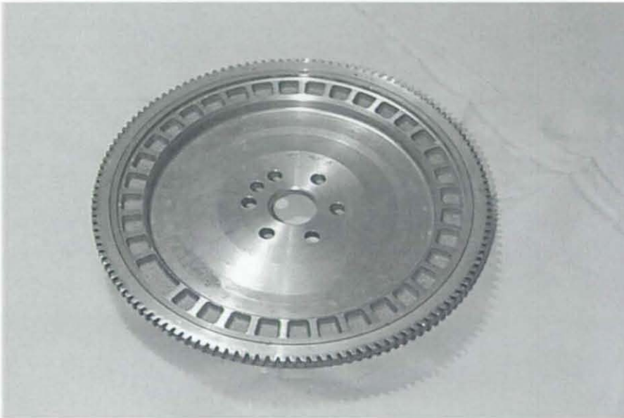
Figure 8.1.10 Flywheel (Cast Iron)
