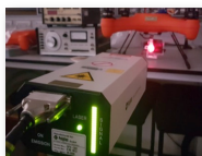
Figure 5 a-b) Camera gimbal self noise using laser Doppler vibrometer
