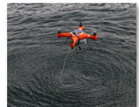
Figure 2) Deployment of hydrophone system from a surface landing UAV
