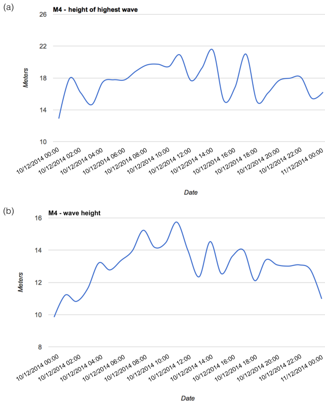
Figure 9. M4 records of (a) maximum wave height (m) and (b) significant wave height (m) on 10 December 2014. Data retrieved from The Marine Institute (2017a).
