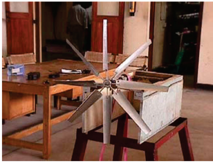
Figure 2. Scale model of rotor 2 and wind tunnel testing facility
