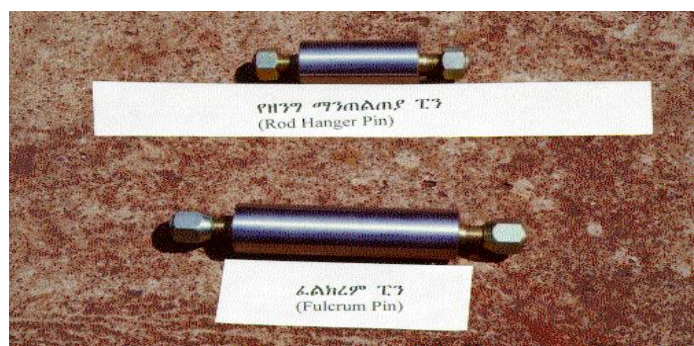
Photograph 3. WEDC – some slow wearing spare parts of Afridev hand pump
