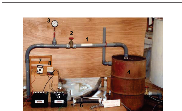
Figure 1. Pump testing system: (1) Delivery pipe, (2) Gate valve, (3) Pressure gauge, (4) Barrel, (5) Batteries, (6) Variable resistor, (7) Ammeter
