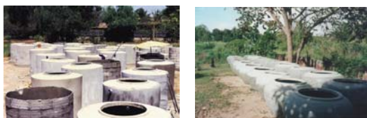
Figure 6. Production of rainwater jar and tanks in the yard of a local private entrepreneur in a village
