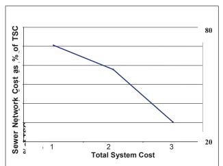
Note: 1=Sewer network + secondary level treatment, 2=Sewer network + secondary + tertiary treatment, 3=Sewer network + secondary + tertiary +advanced (ultra-filtration + RO + UV) treatment
