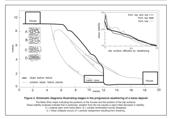
cohesion. Figure 2 indicates that slopes which, in an unweathered state, have safety factors close to unity might fail after only a short period of progressive weathering. This process will take considerably longer for the initially more stable slopes. Within the urban environment the man-made cut slopes are frequently close to equilibrium and therefore moderate amounts of weathering affected by *e.g.* the uncontrolled disposal of waste water may bear great risks for these sites.
