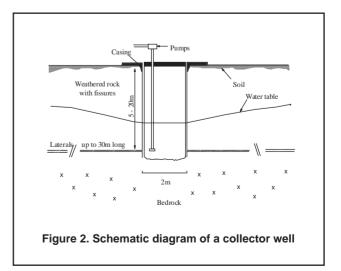
L s-1 for slim boreholes at pumping drawdowns in excess of 30 m (Wright, 1992).
