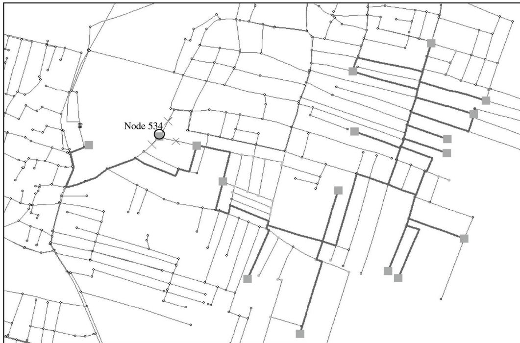
Figure 9. Alternate path for water flow to nodes bypassing the contaminant affected node (534).
