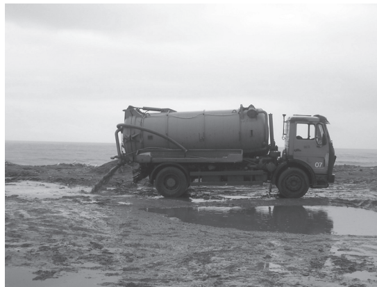
Photograph 1. Tanker discharging faecal sludge at Korle Gono
