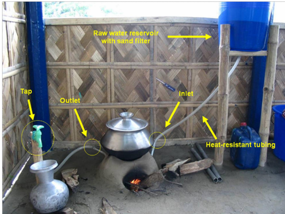
Photograph 1. Chulli system components
