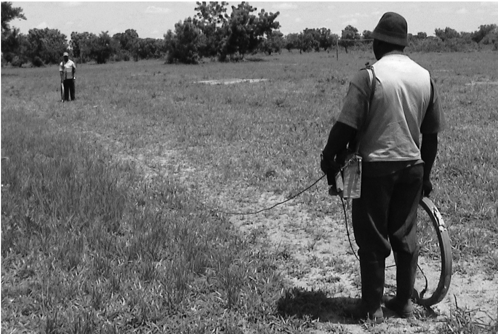
Photograph 6.2. Electromagnetic survey to locate water-bearing fractures
