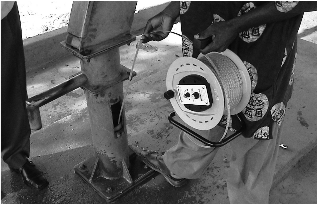
Photograph 9.1. Monitoring groundwater levels in Ghana
