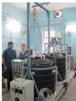
Photograph 1. 600L ECAR batch reactor prototype at Jadavpur University
