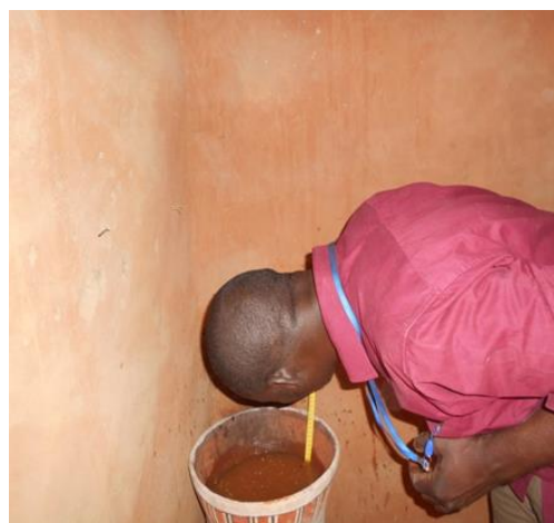
Photograph 2. Mr. Boubacar of SP Niger checking the height of the biolayer
