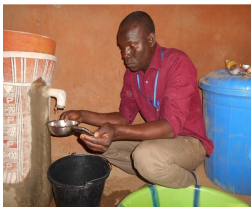
Photograph 1. Mr. Boubacar of SP Niger conducting a flow test during the pilot testing of the clay-bodied BSF
