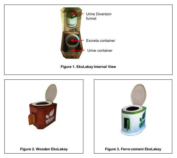
Whereas the more expensive wooden toilet model allows for easy repairs by SOIL technicians and has been deemed more attractive by some customers, the lower cost ferro-cement model is more durable and better suited to contexts where flooding is a concern.
