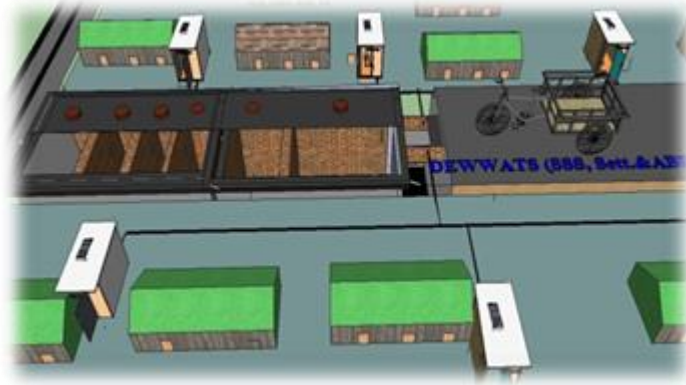
Figure 1. Model of SBS and Settler with ABR
