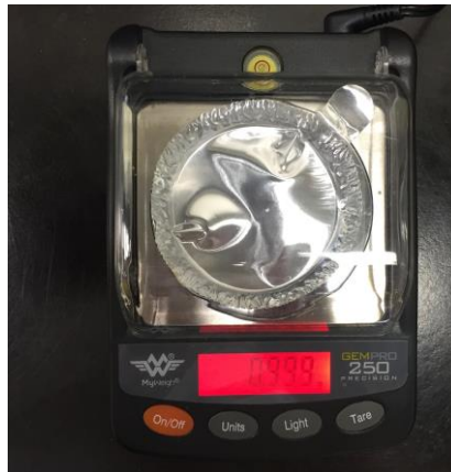
Photograph 2. Scale B with a 5 cm aluminium weighing dish completely covering its weighing plate
