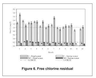
The high consumption of the residual chlorine within the plant premises and distribution reservoirs is a good indication (Figure 6) that water might reach the furthest consumer point without enough residual chlorine. Free chlorine in the three distribution reservoirs at Muyenga, Naguru, Rubaga and Mutungo were 0.45, 0.15, 0.15 and 0.10mg/l while the corresponding total chlorine concentrations were 0.80, 0.55, 0.50 and 0.45 mg/l respectively.
