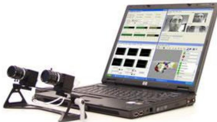
**Figure 2-20: non-intrusive eye tracking equipment (desk mounted)**
