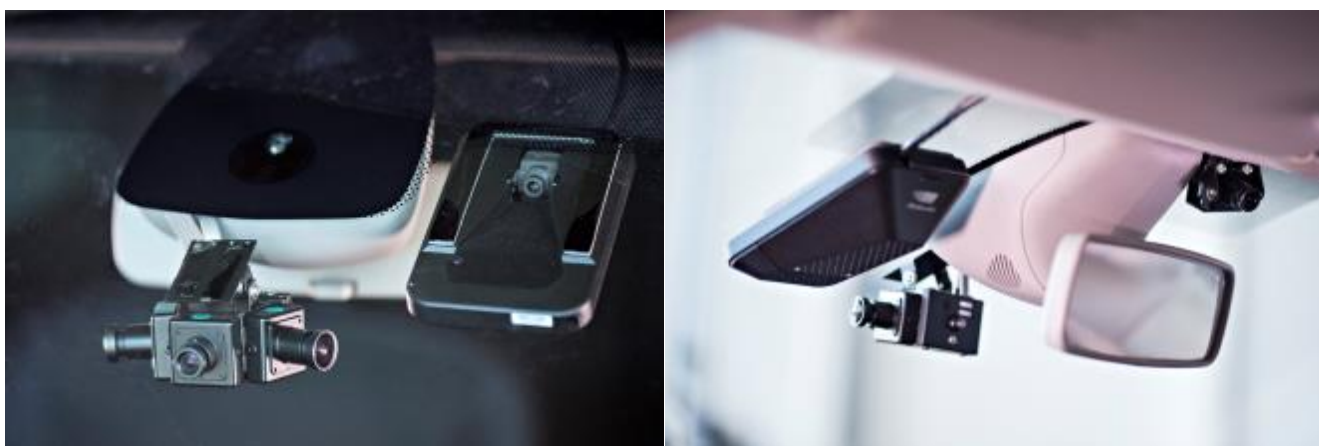
Figure 6 and Figure 7: Forward cameras and MobileEye (left) as well as driver compartment camera (right) in a UK car installation
