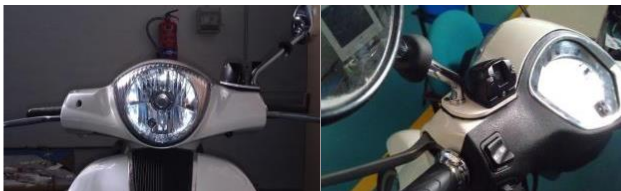
Figure 21 and Figure 22: PTW forward (left) and driver face (right) cameras
