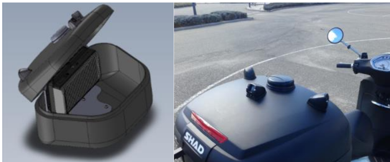
Figure 19 and Figure 20: Topcase for PTWs, showing the DAS, 3 cameras and GPS antenna
