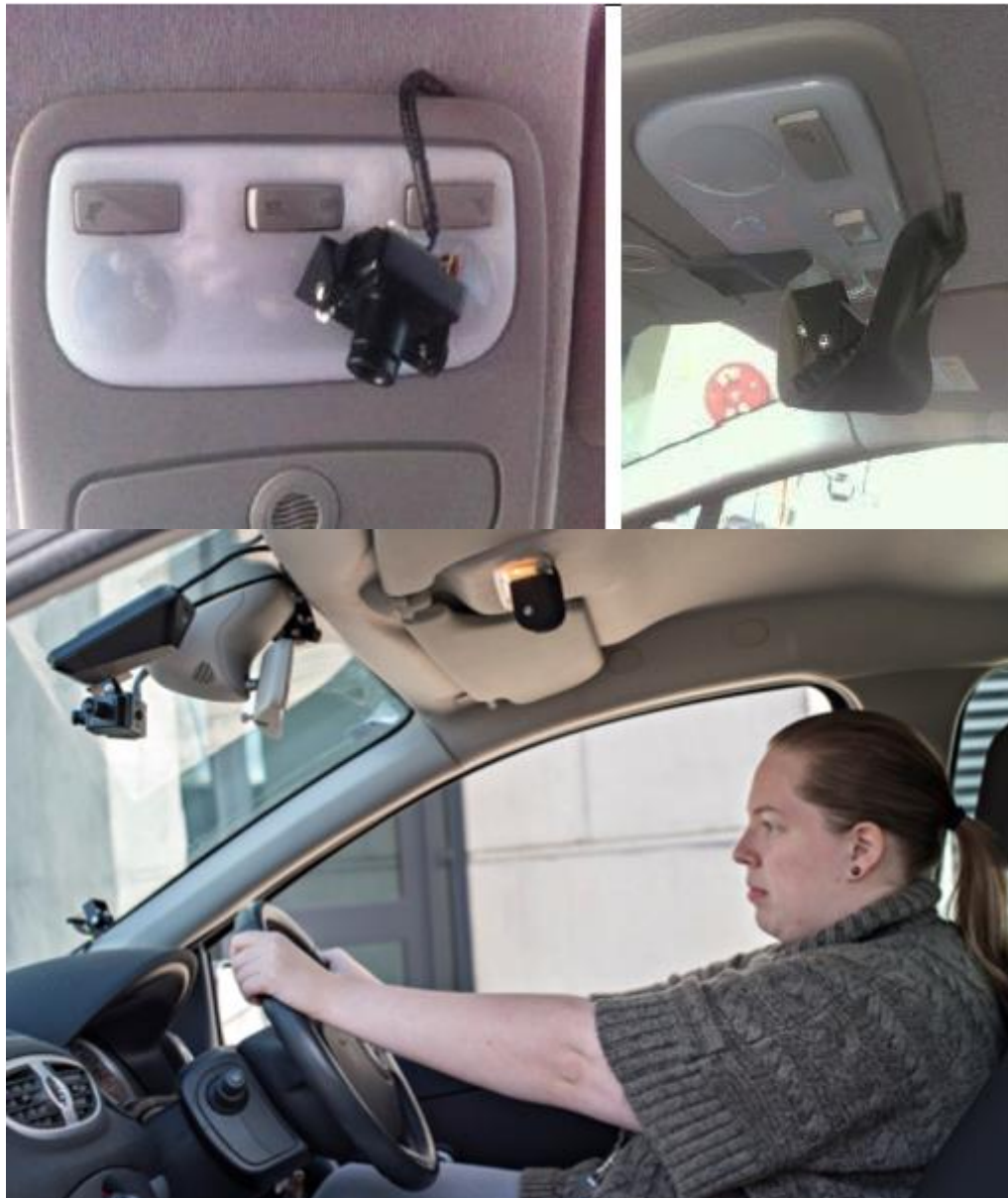
Figure 8 and Figure 9: Ceiling camera and cover protection clipped onto it after setting as well as driver face camera along windshield pillar in a UK car installation
