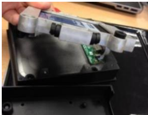
Figure 24: DAS Hard drive protection system, relevant for change of hard drive
