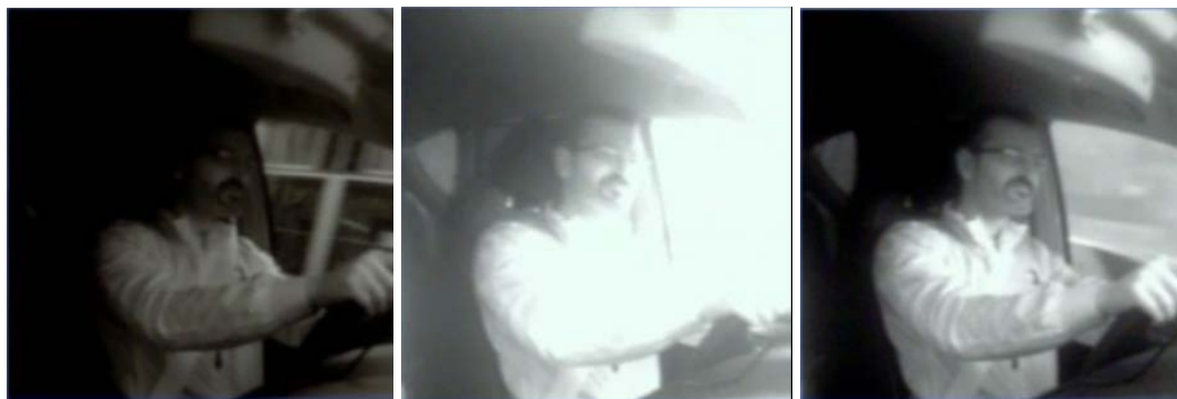
Figure 2-8: Video frames showing under/over exposure
