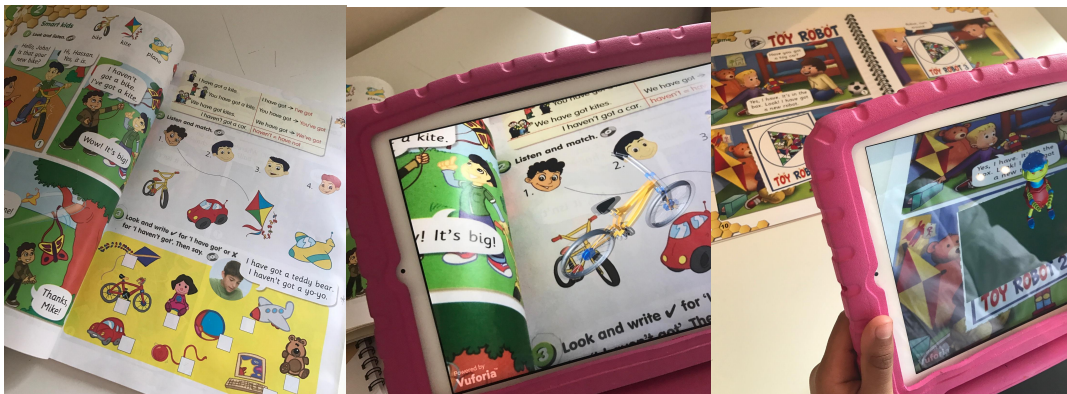
Figure 14: The images in the textbook as AR markers, and the AR scene based on the printed content of the textbook.
