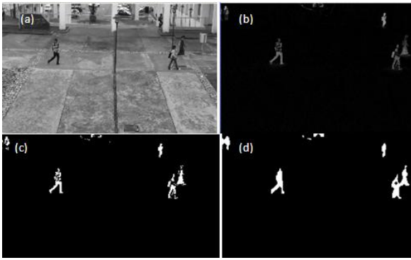
Figure 4. (a) Input video image (b) Background subtraction (c) Autothreshold (d) Dilation and Erosion.
