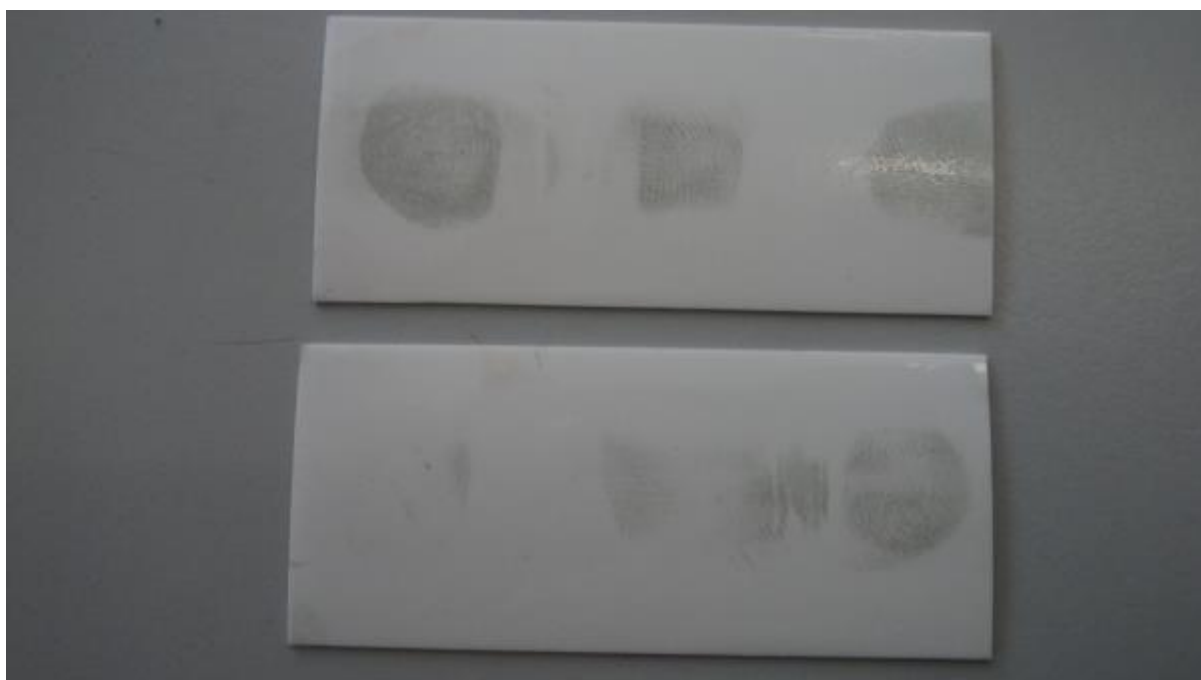
Figure 31 - Contact with a copper pipe for 10 seconds (top) and 1 second (bottom)
