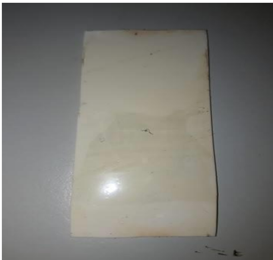
Figure 82 - Blue/black colour forms on surface of gel (myristic acid)
