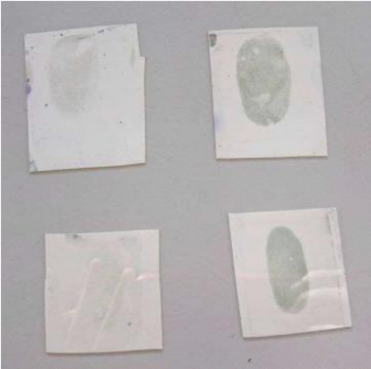
Figure 73 - Comparison between desiccated prints (right) and non-desiccated (left) at 24 hours (top 2) and 48 hours (bottom 2)
