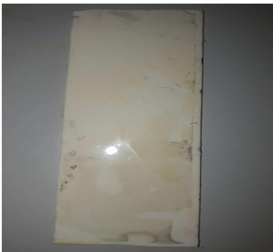
Figure 82 - Blue/black colour forms on surface of gel (myristic acid)
