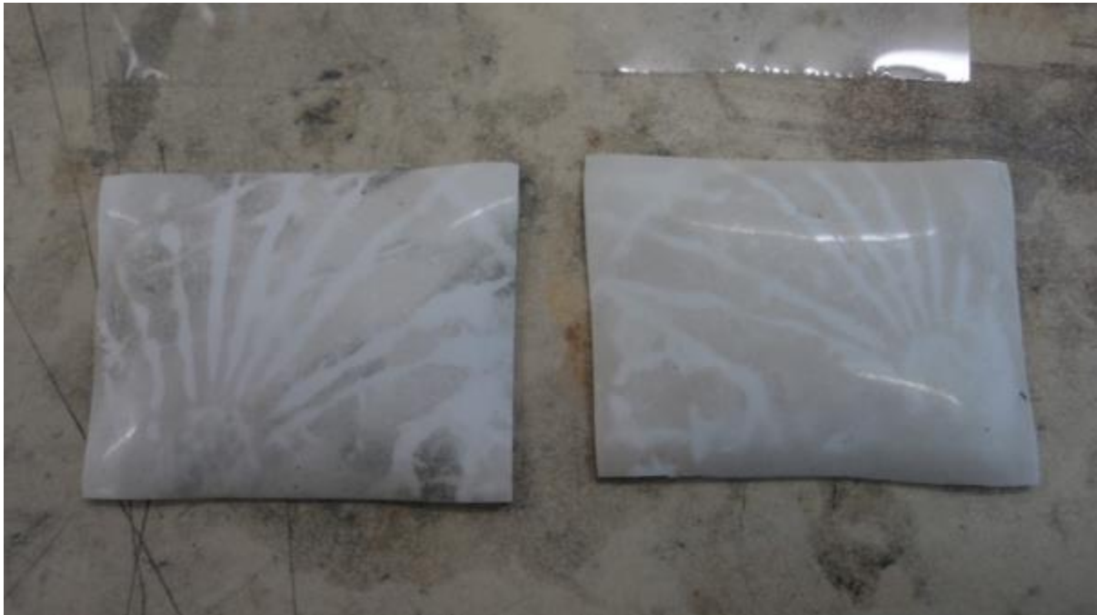
Figure 45 - Copper from sole of shoe on the left, in contrast to no copper on the right.
