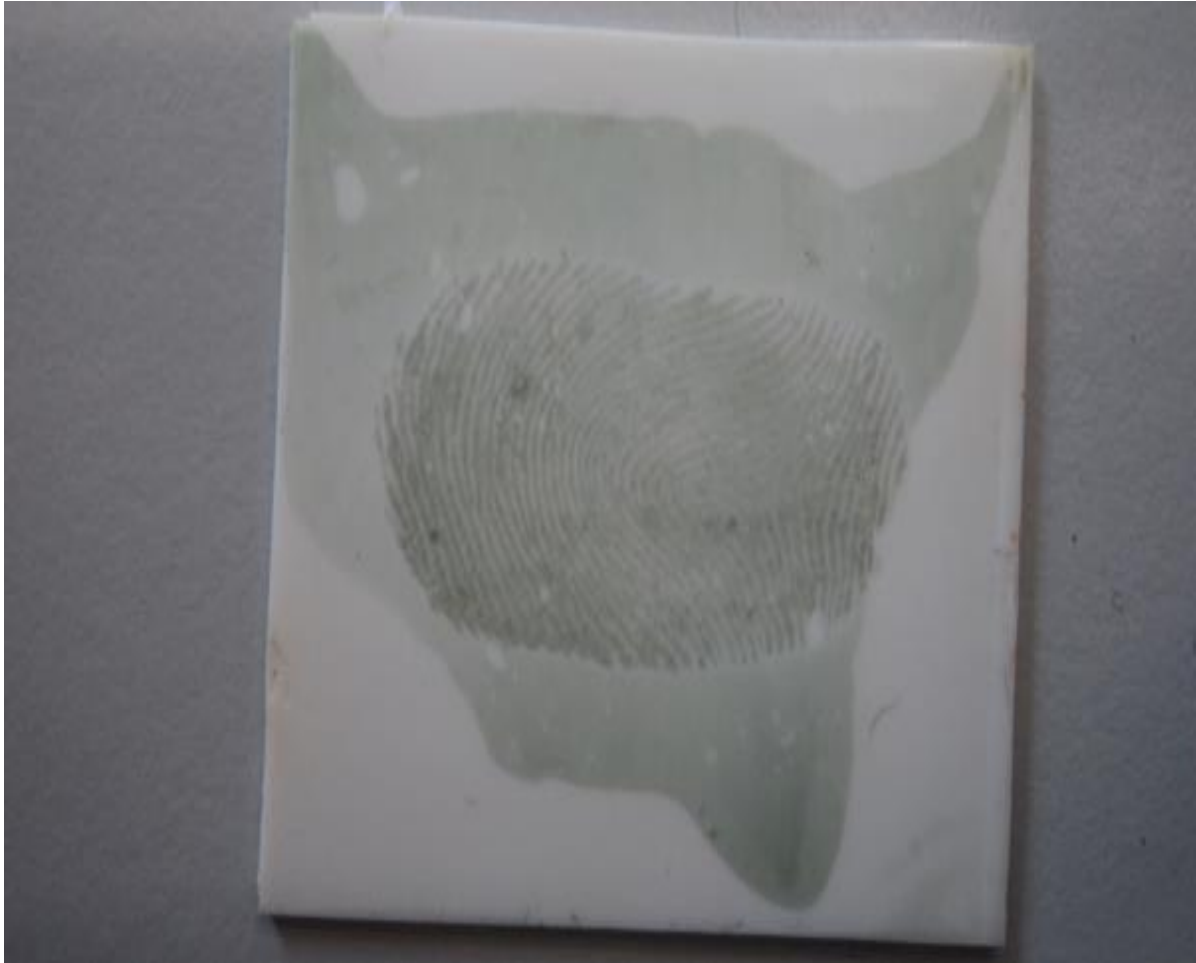
Figure 55 - An example of how background can affect fingerprint visualization even when there is a good quality fingerprint
