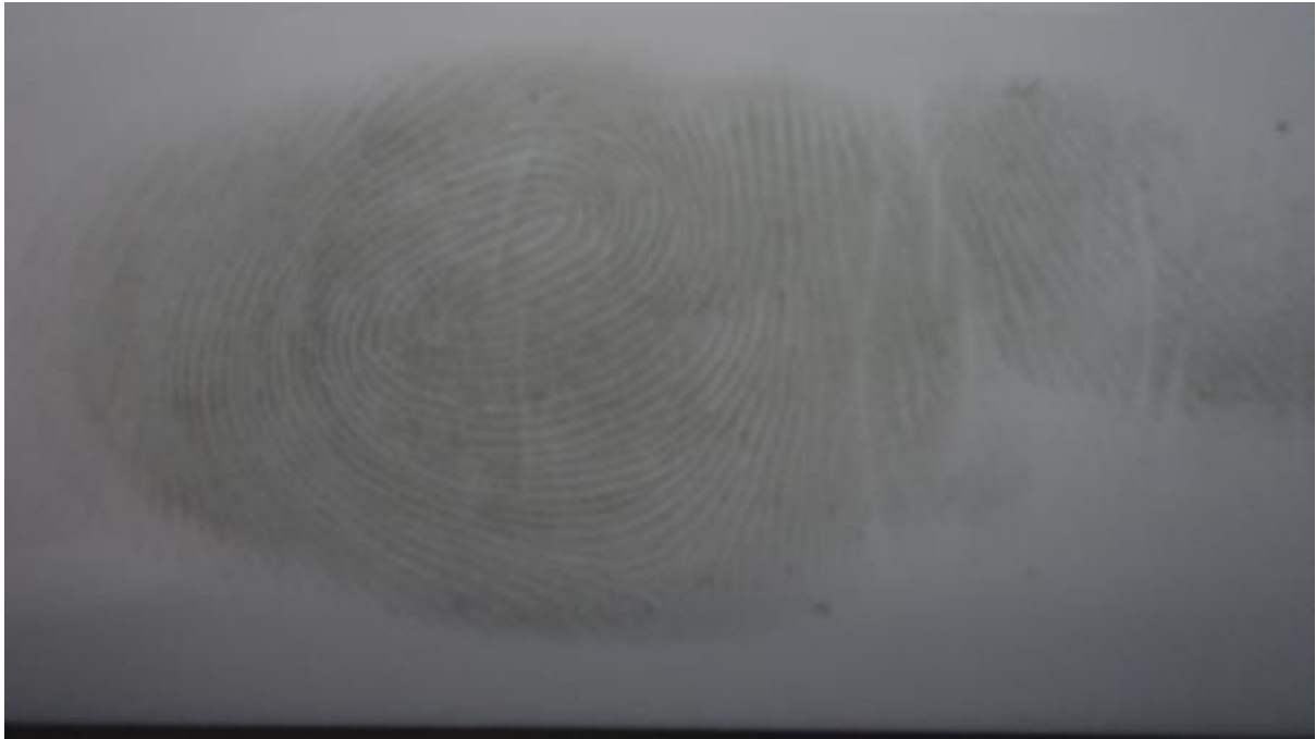
Figure 50 - Excellent detail that can be obtained from the surface of the skin via rubanic acid development from copper
