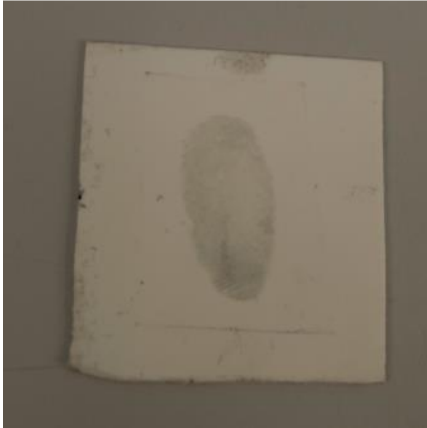
Figure 88 – Fingerprint developed from stainless steel
