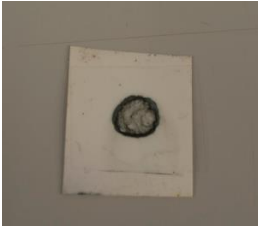
Figure 76 – Proof that amino acid is reacting with rubeanate solution
