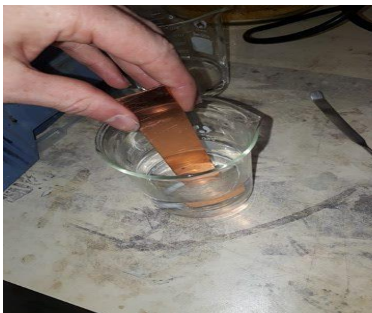
Figure 80 - Copper placed in solution of fatty acid
