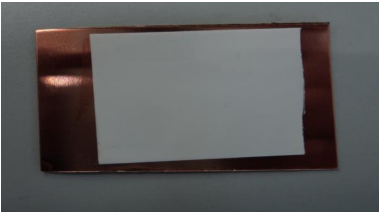
Figure 53 - Gelatine lifter placed over the fingermark on the copper
