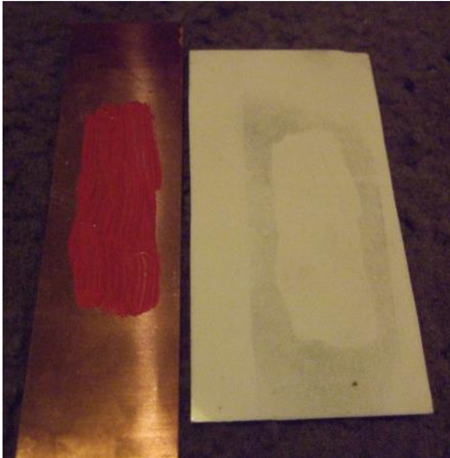
Figure 21 – The area covered by paint on the copper (left) is then visualised in the development using rubeanate solution
