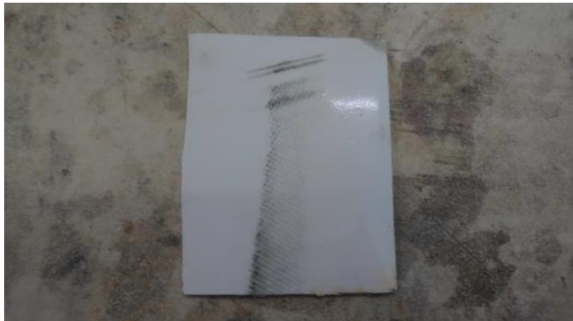
Figure 42 - Copper traces lifted from polyester rucksack. There is slight detail of the design itself also shown
