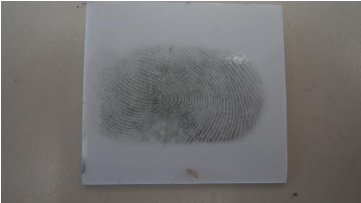
Figure 47 - Copper sheet handled for 1 minute
