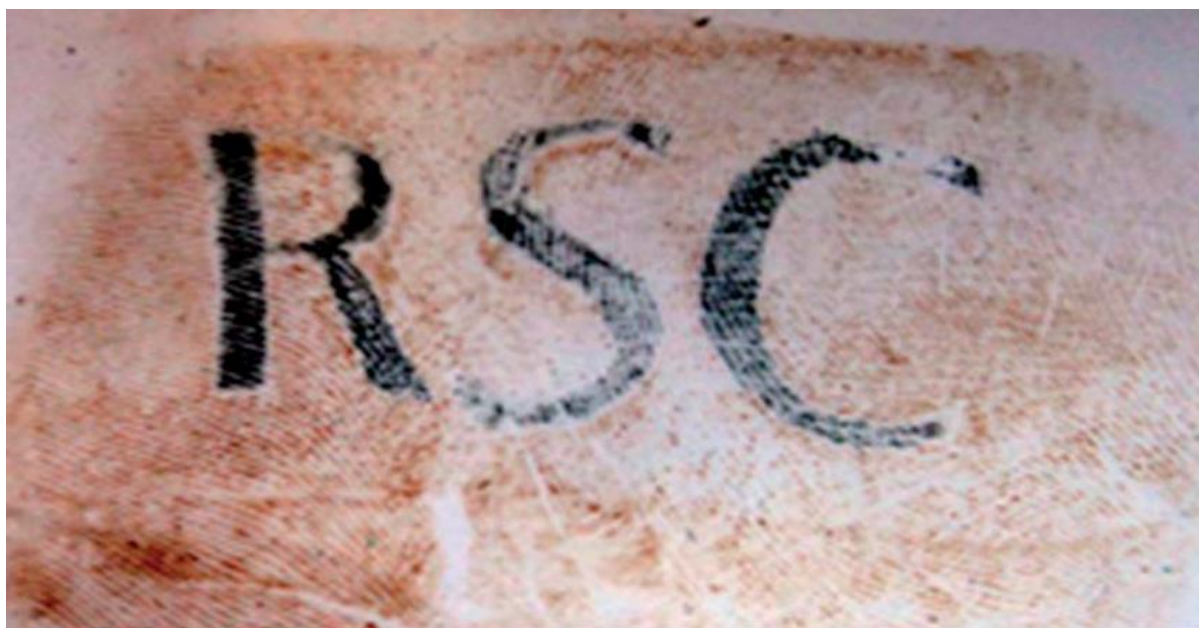
Figure 22 - The blue black of copper is apparent with the RSC, against a backdrop of orange/brown from the lead block.
