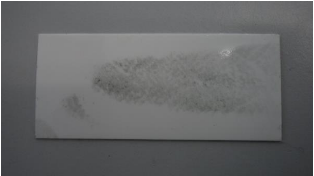
Figure 40 - Copper detected on surface of a woolen glove used to handle copper
