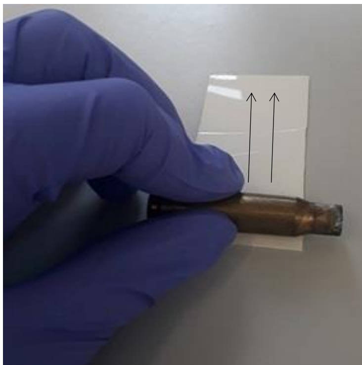
Figure 85 - 'Rolling' casing across the gelatine lifter
