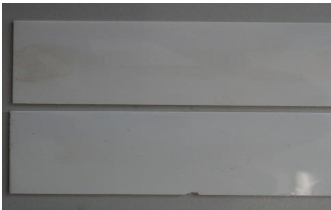
Figure 32 – (Top) After 10 seconds of contact time with lead, there is evidence of lead rubeanate formation, however after 1 second (bottom) there is not.
