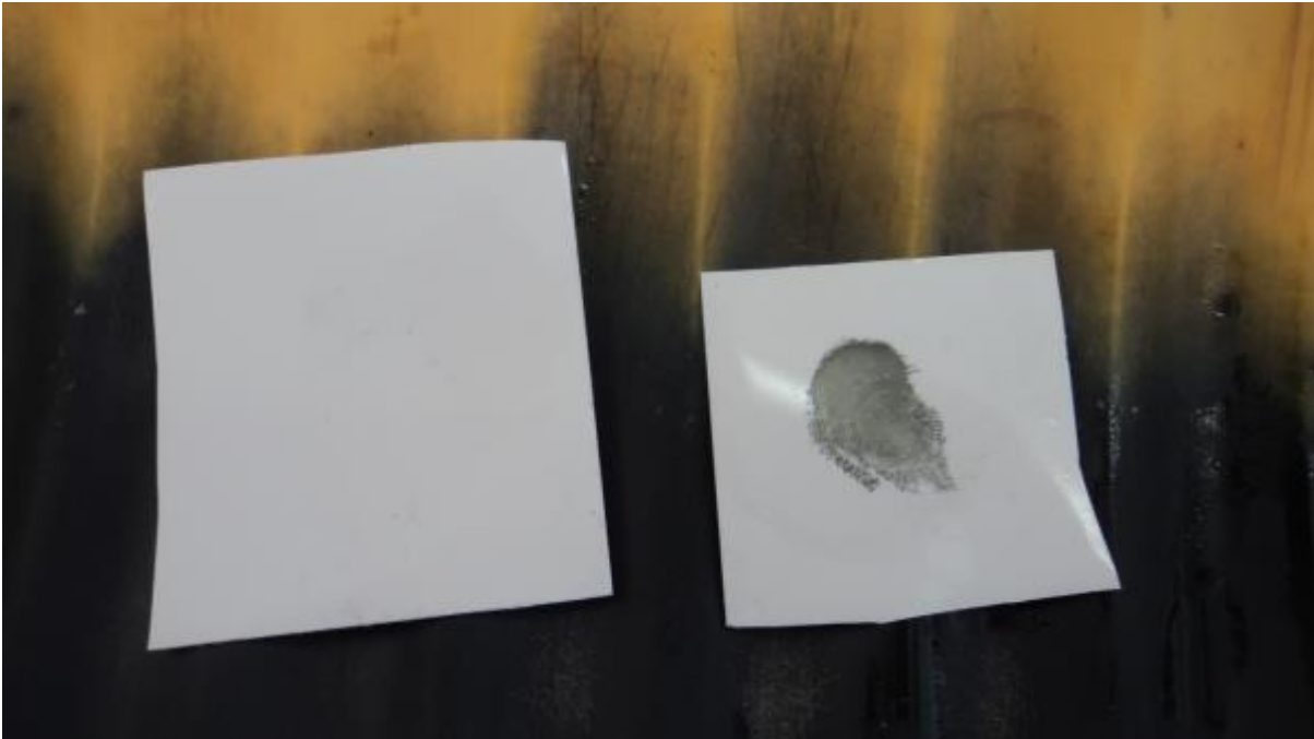
Figure 19 - Hand rinsed after contact with copper sulphate (left), differed considerably to when not rinsed (right).
