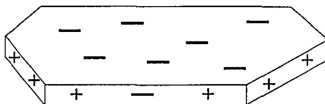
Figure 6.2 : Sketch of a typical kaolin crystal
