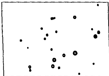
(4) Open : Removes noise on image. This function is a combination of Erode then Dilate (Set-3 iterations)
