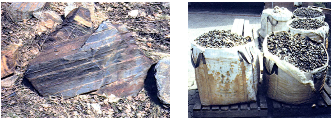
Fig. 4. Sulfide seams in rock samples: a) detail of slate and b) aggregate for testing.
