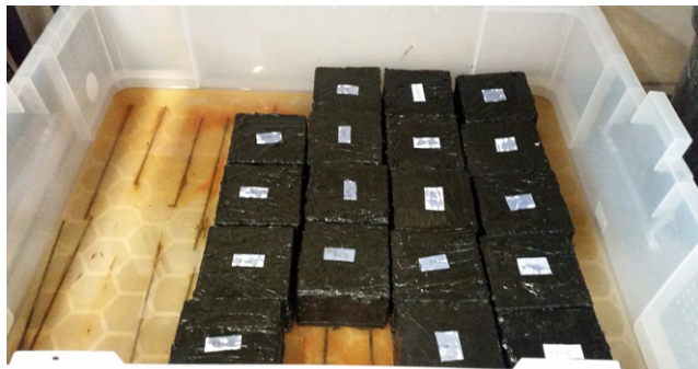
Figure 4. Cubes exposed to chloride-ion solution by the inversion method
