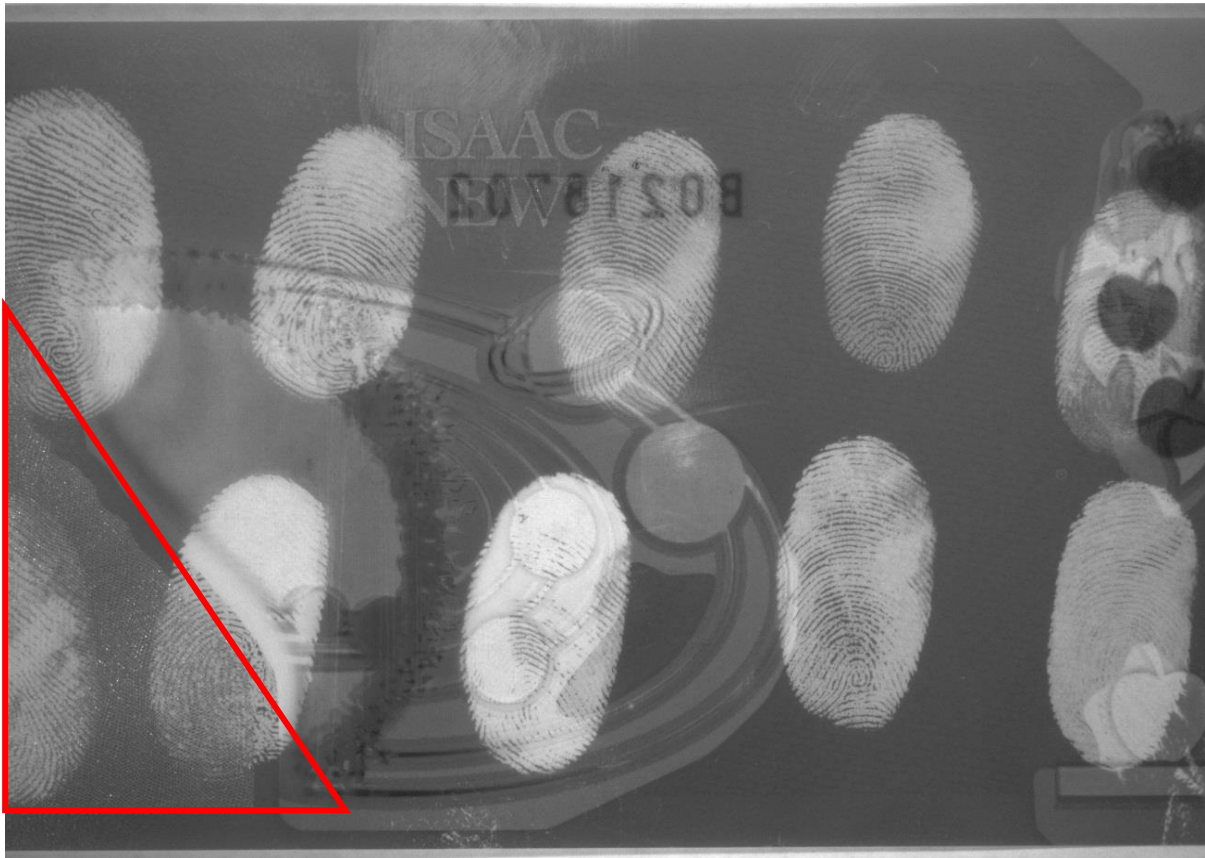
Figure 127: NT Cu VMD (3.0 nm Thickness) Treated Polymer Banknote Viewed with Reflected IR (B&W)
