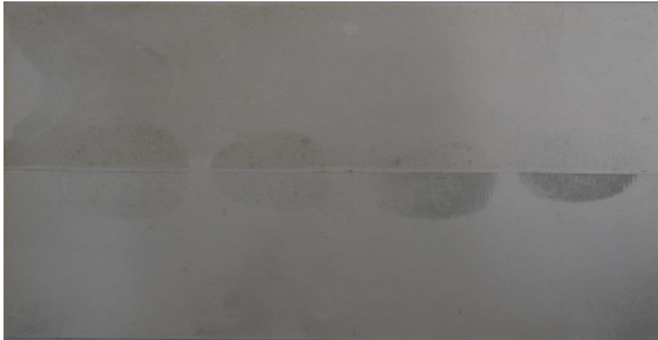
Figure 92: Gel Lift from Copper 4 th Use after 3 rd Clean
