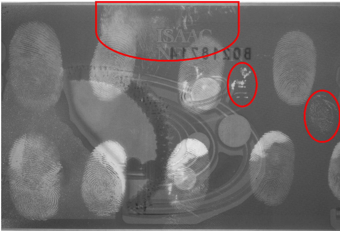
Figure 119: NT Cu VMD (2.1 nm Thickness) Treated Polymer Banknote Viewed with Reflected IR (B&W)
