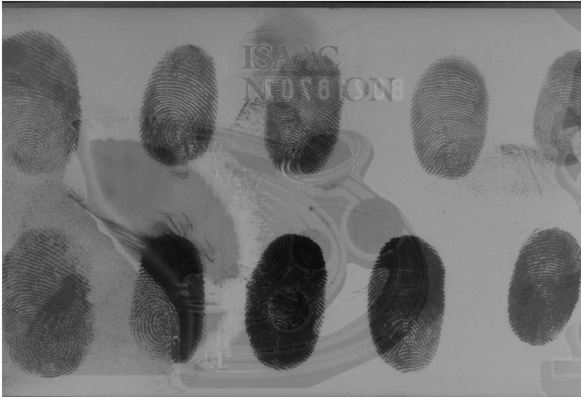
Figure 128: NT Cu VMD (3.0 nm Thickness) Treated Polymer Banknote Viewed with Reflected IR - Inverted (B&W)
