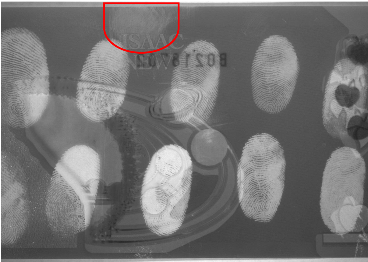
Figure 130: Bare Cu VMD (2.1 nm Thickness) Treated Polymer Banknote Viewed with Reflected IR (B&W)
