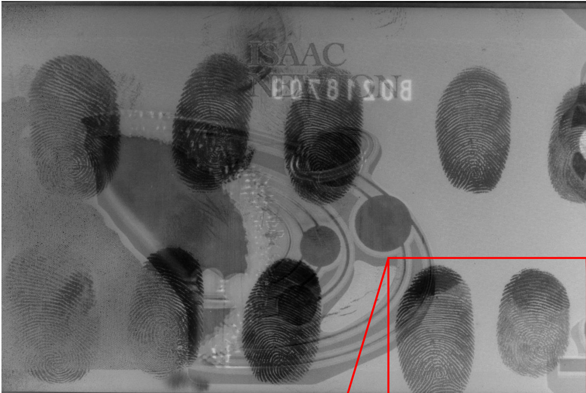
Figure 124: NT Cu VMD (2.5 nm Thickness) Treated Polymer Banknote Viewed with Reflected IR - Inverted (B&W)*
