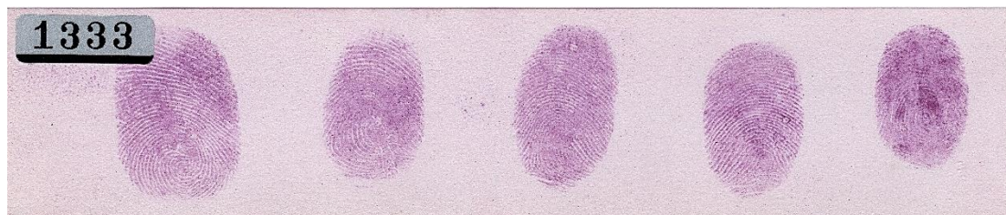
Figure 50: Ninhydrin Development via Humidity Chamber
