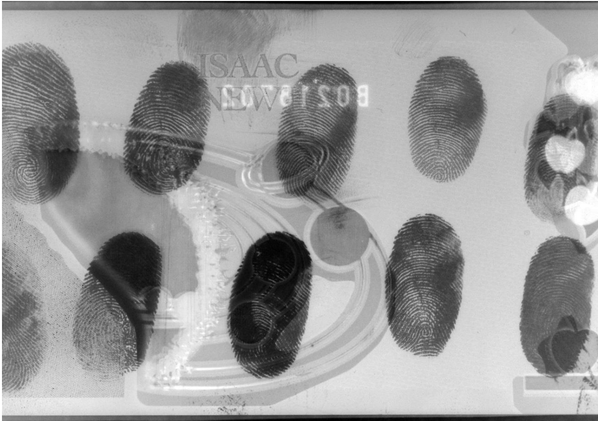
Figure 131: Bare Cu VMD (2.1 nm Thickness) Treated Polymer Banknote Viewed with Reflected IR - Inverted (B&W)
