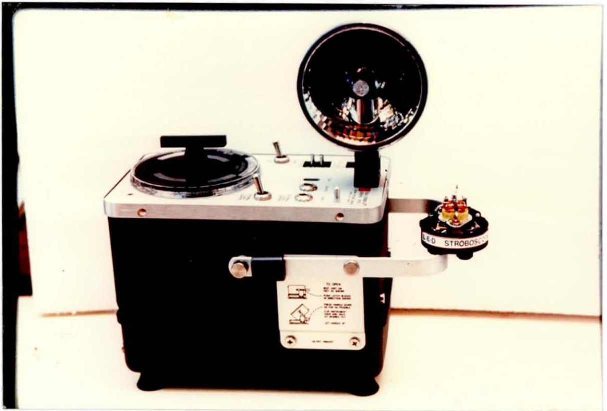
Fig.9.10 THE LED STROBOSCOPE ON THE HANDLE OF THE STROBOTAC
