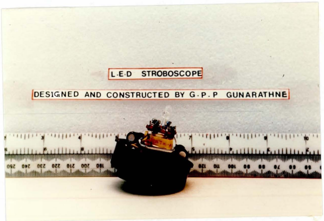
Fig. 9.9 THE LED STROBOSCOPE ASSEMBLED IN A LENS CAP READY TO BE LOCKED IN TO THE OPTICAL ASSEMBLY.
