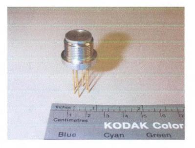
Figure 4.1 Picture of 4000PSI rated Pressure Transducer
