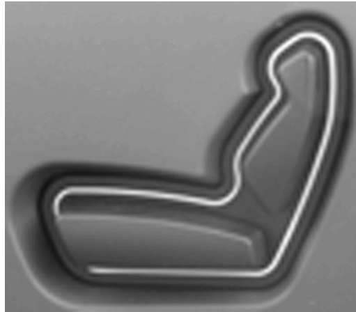
Figure 2. A seat adjustment control which exhibits excellent natural mapping or matching between the system and the user's mental model.
