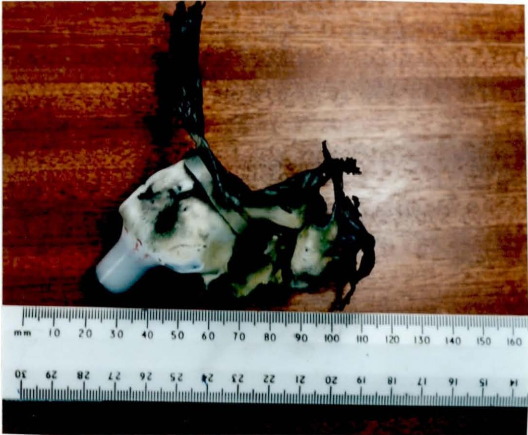
Figure (8.3d) Tested HDPE ring of 17.55 mm o.d, and 13.75 mm i.d placed on an HDPE cylinder of 13.75 mm o.d fired by an 8cm/22swg wire at 25 kV.
