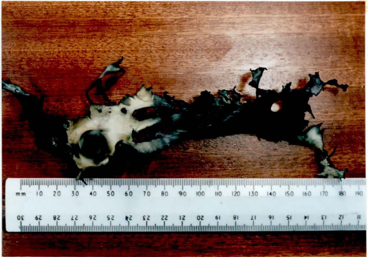
Figure (7.4d) Fractured HDPE tube, 13.56 mm o.d., and 3.5 mm thick fired by an 8cm/22swg wire at 25 kV.
