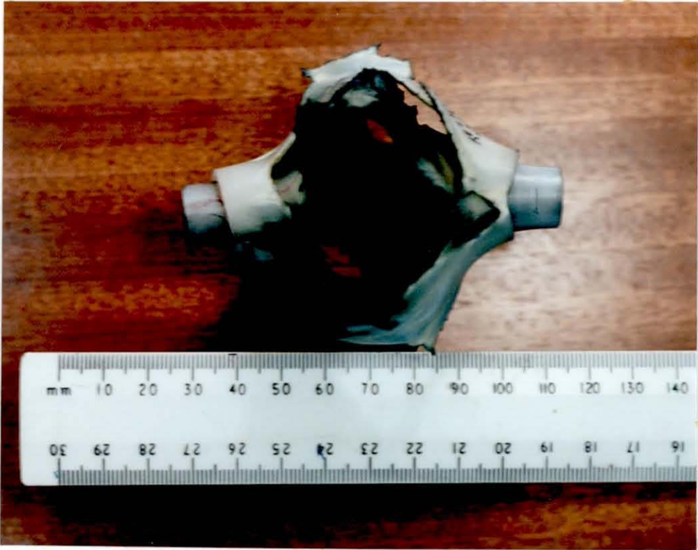
Figure (7.6d) Double HDPE tubes fractured by an 8cm/22swg wire explosion at 25 kV.
