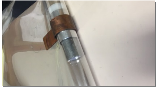
Figure 5. Magnetic implosion assembly during the preparations for a shot. The sacrificial copper coil has the imploding samples for cold welding mounted inside.
