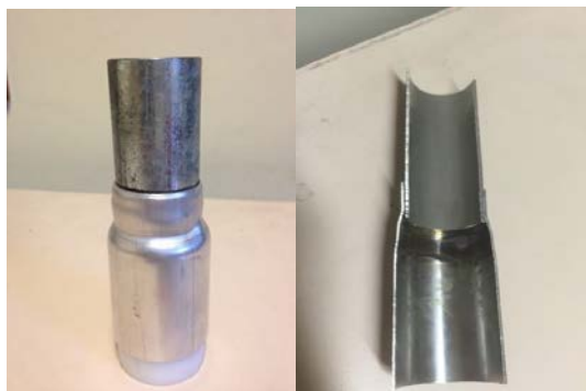
Figure 10 Typical cold welding of stainless steel cylinders.
