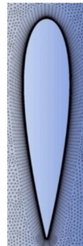
c. Structured mesh in the boundary layer region
