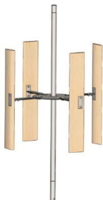
Figure 6. 3D geometric model of the H-Darrieus turbine
