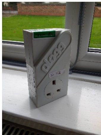
Figure 14 - Electricity meter logger plug
