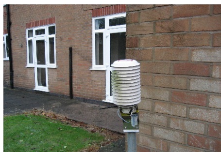
Figure 19 - Naturally aspirated radiation shield for external air temperature monitoring
