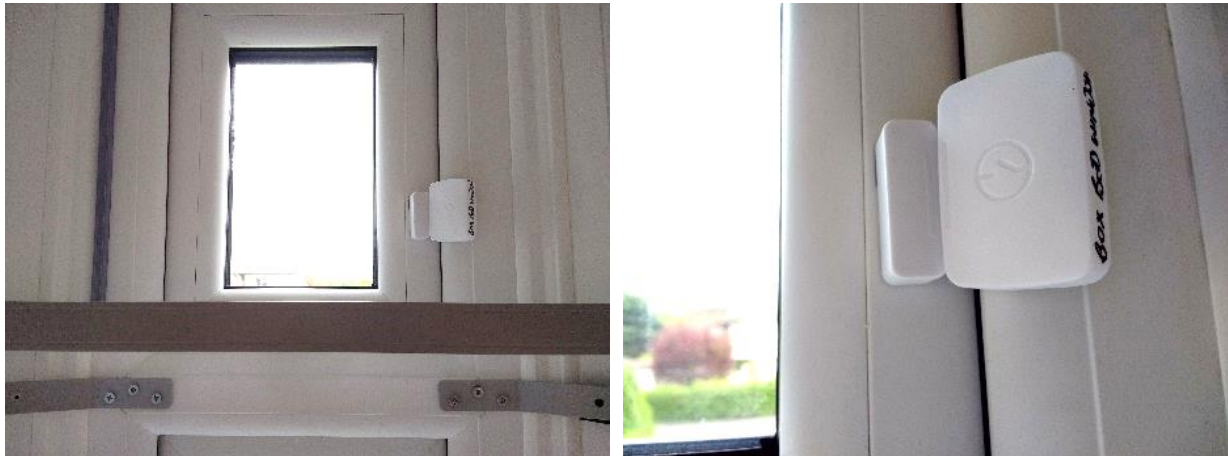
Figure 13 - A contact sensor used to record window opening status was wirelessly connected to the smart home controller and status logged
