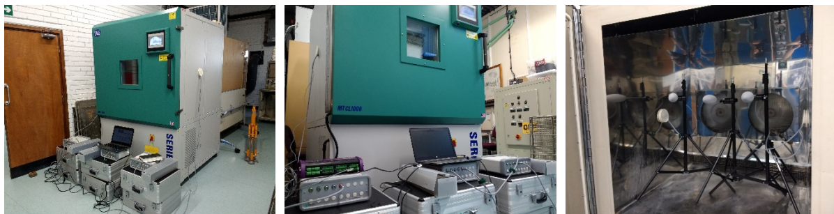
Figure 18 - Calibrating operative probes in a climate chamber using a previously calibrated U-type thermistor
