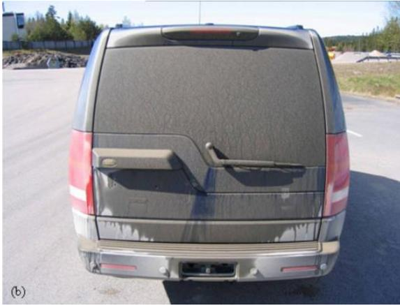
Figure 2. Deposition image for a SUV from a wetted gravel test track [7]
