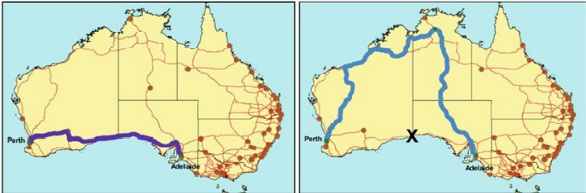
Figure 2.8. The diversionary route following a low probability flood event on the Eyre Highway, Australia after D’Este and Taylor (2001).
