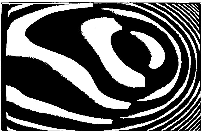
Figure 2.6: (a) Fringe pattern. (b) and (c) Sign inversion after the Fourier transform method applied along the horizontal and vertical directions respectively.
