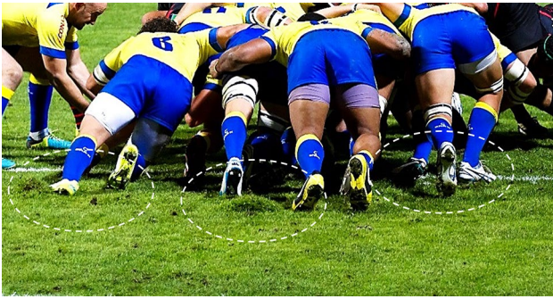
Fig. 1 Photographic evidence of natural turf system damage caused by the back row of a rugby scrum
