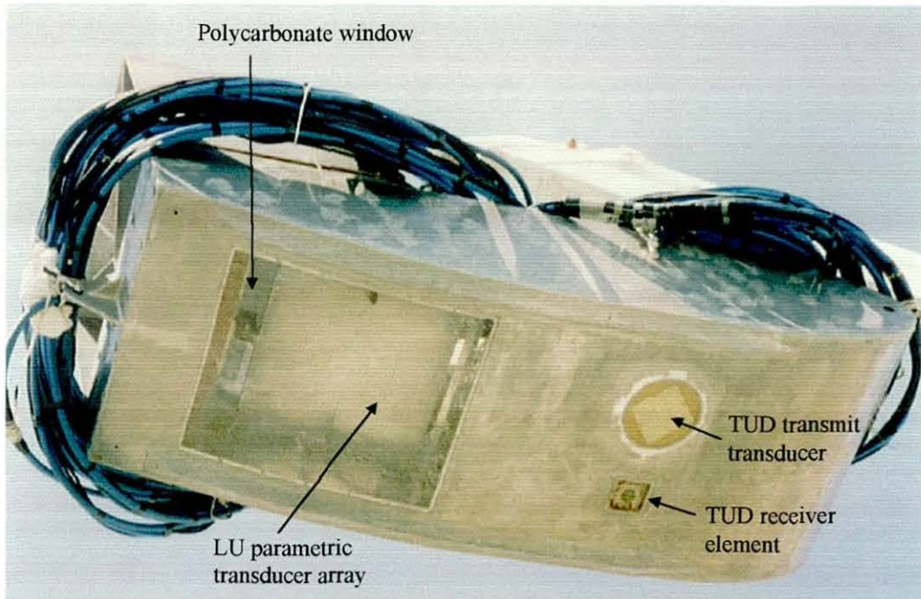
FIGURE 6.3 REBECCA PROJECT TOW-FISH UNDERSIDE VIEW
