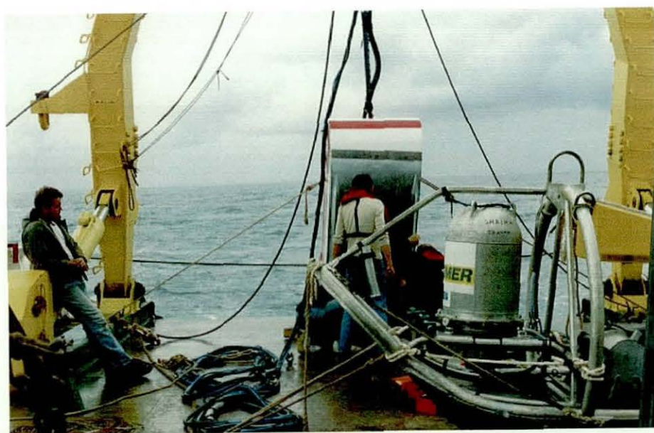
FIGURE 6.5 ACOUSTIC TOW-FISH DEPLOYMENT AND SHRIMP SYSTEM
