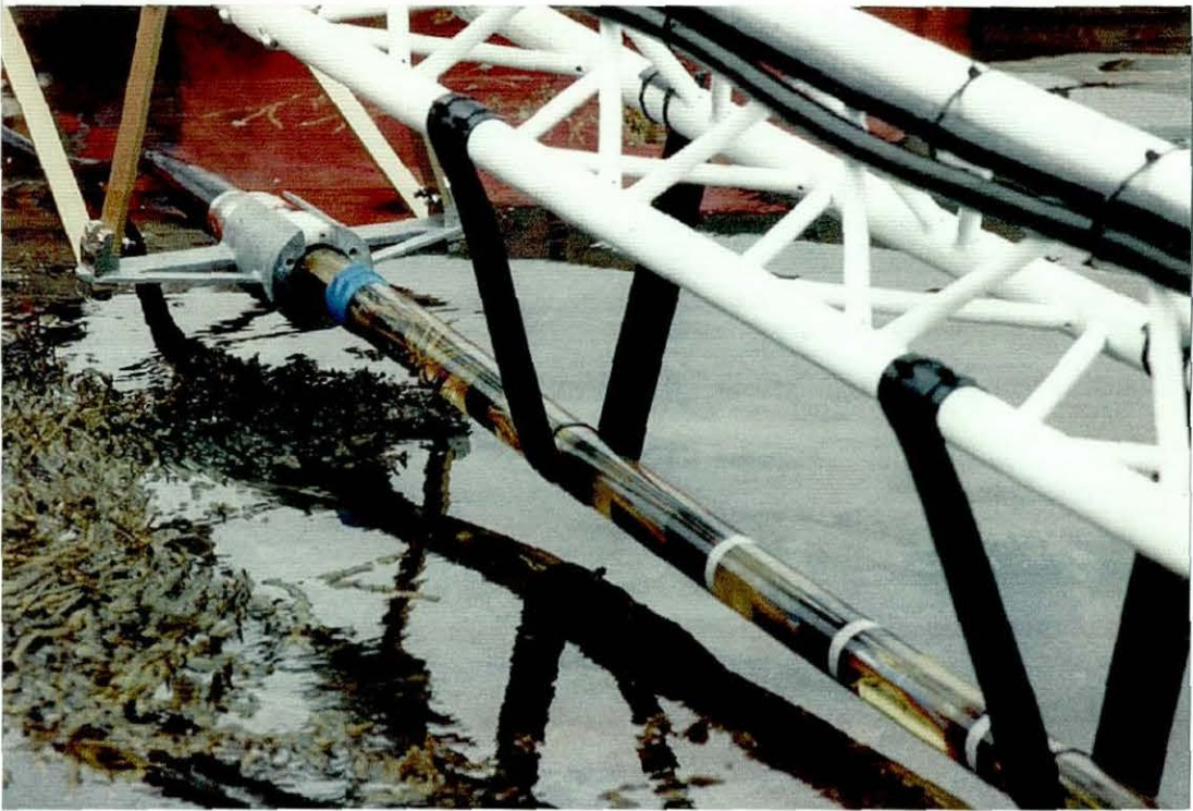
FIGURE 7.7 STREAMER ARRAY, HORIZONTAL DEPLOYMENT FOR BOTTOM-SCATTERING MEASUREMENTS
