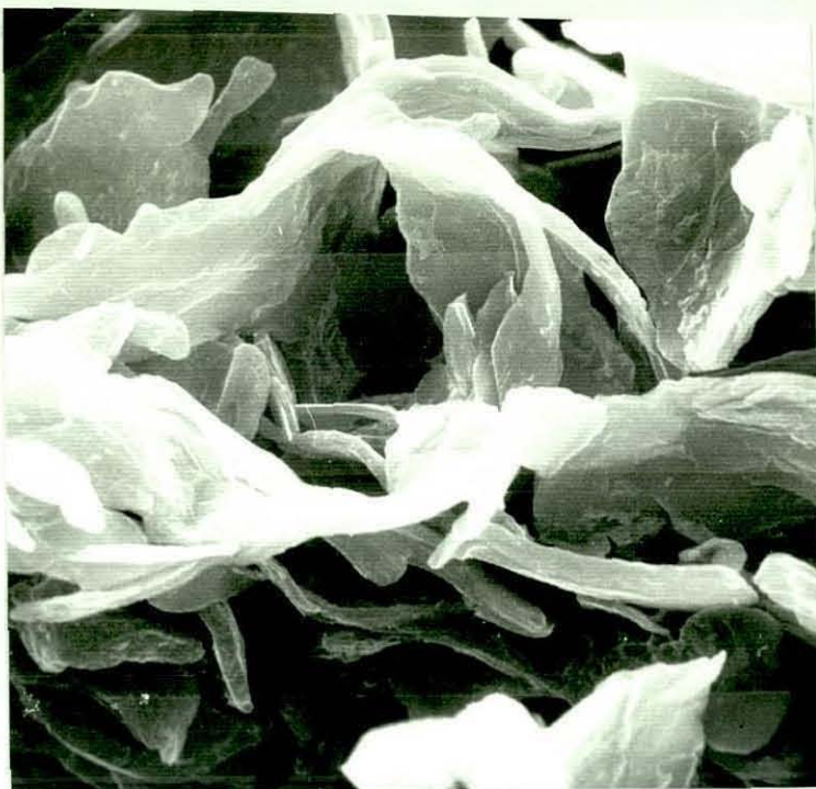
Figure 36 Flake Graphite Modified by Melt Treatment with 0.016% Ce MM and 0.16% Ca, Deep Etched (Casting 1/6)
