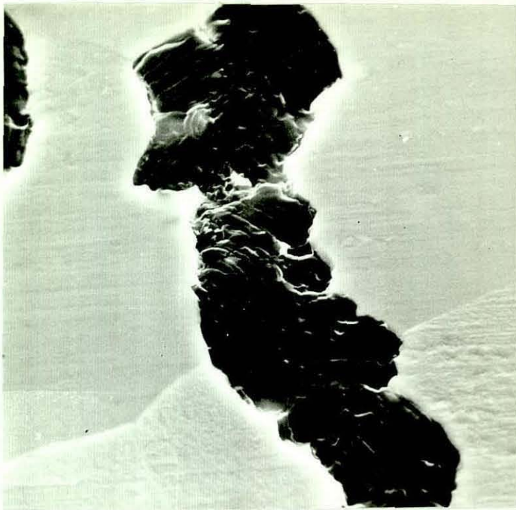
Figure 56 Compacted Graphite: Change in Orientation of the Basal Plane Traces at the Growth End of Compacted Graphite (casting 1/14).
