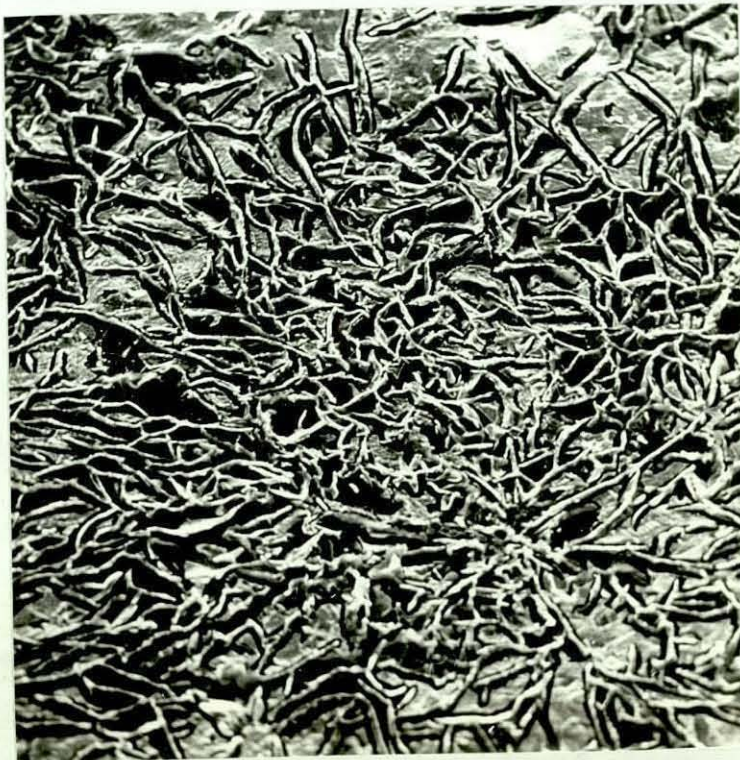
Figure 35 ASTM Type D Flake Graphite, Deep Etched (Casting 2/6)
