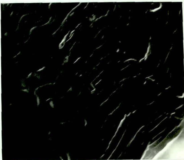
Figure 53 Nodular Graphite: Change in the Orientation of the Chevron Pattern at the Nodule Periphery (casting 1/14).
