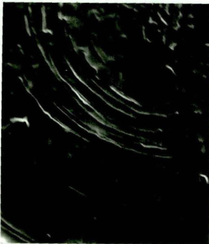
Figure 49 Nodular Graphite: Concentric Ring Pattern Produced by Ion Etching (SEM image) (casting 1/14).
