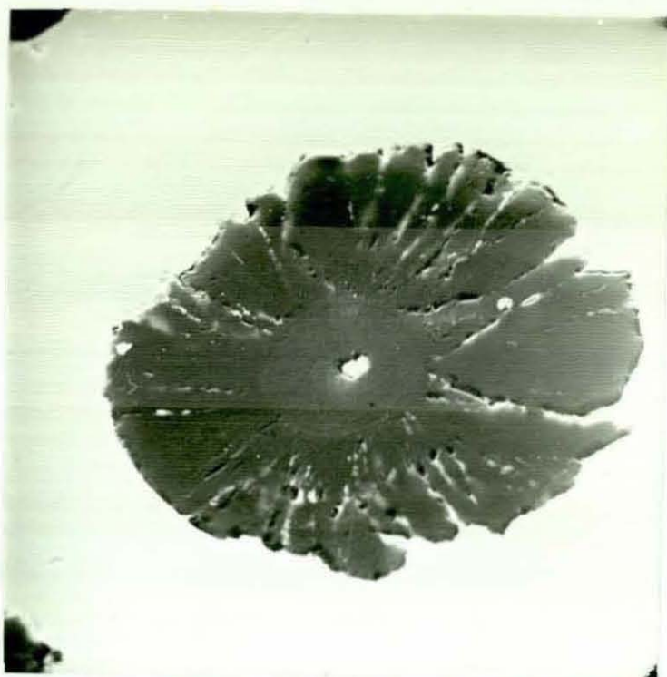
Figure 69 Graphite Nodule in Iron B Showing Centrally Located Inclusion (SEM image)
