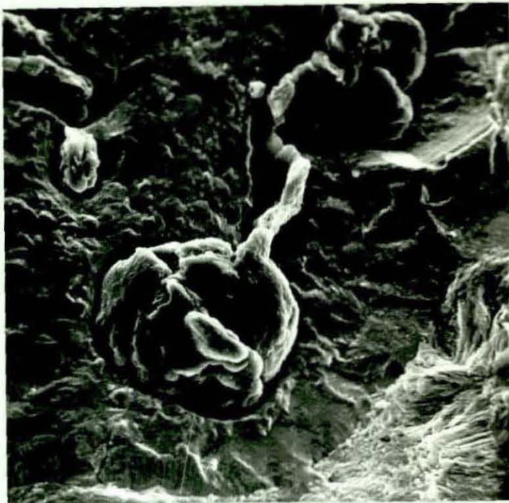
Figure 58(c) SEM Image of a Hybrid Nodular/Compacted Graphite Particle (casting 2/3).
