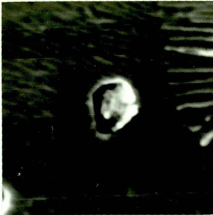
Figure 85(a) Rare-earths Bearing Particle in Iron B, Analysed Using Energy Dispersive X-ray Microanalysis (See Figure 85(b)) SEM Image
