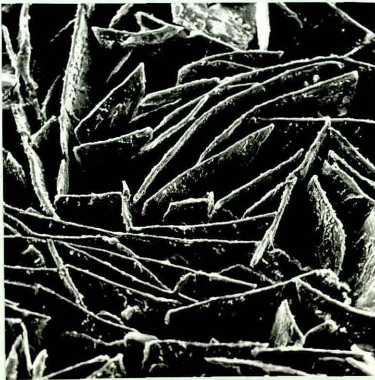
Figure 33 ASTM Type A Flake Graphite, Deep Etched (Casting 2/5)
