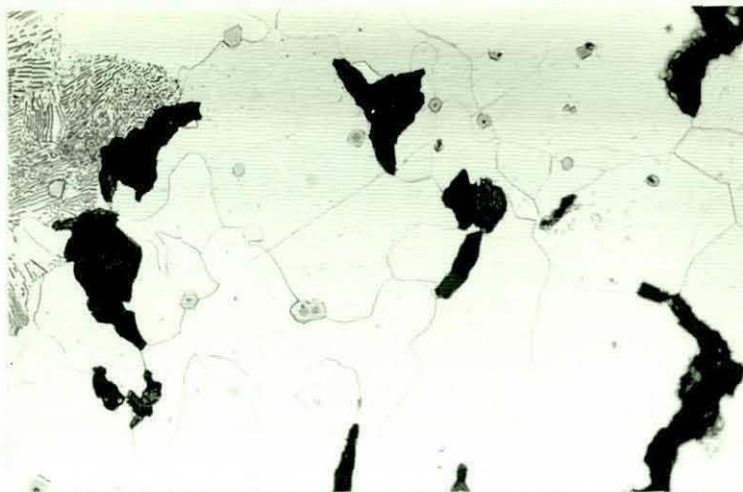
Figure 95 Optical Micrograph of Iron J, Showing Duplex Zirconium-Titanium Inclusions
