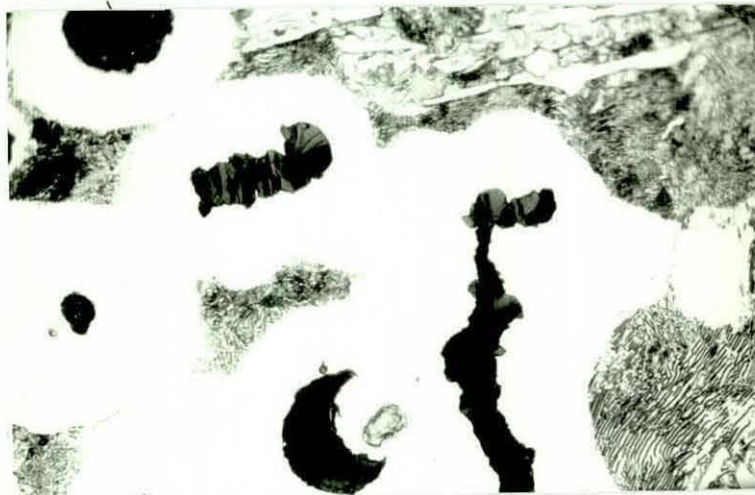
Figure 47 Birefringence Patterns in Compacted Graphite (casting 2/10).
