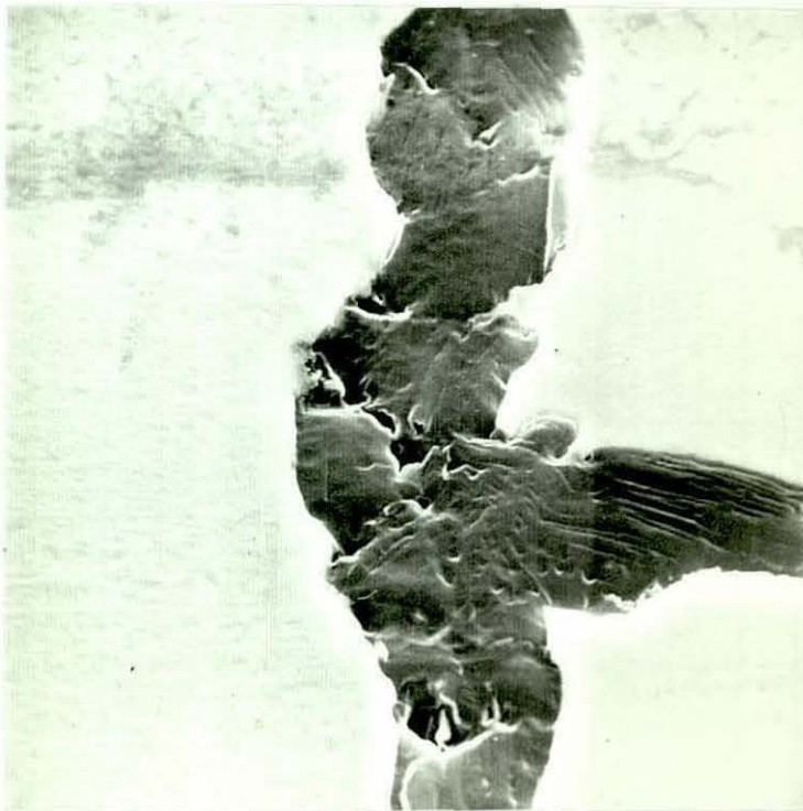
Figure 57 Compacted Graphite: Change in Orientation of the Basal Plane Traces at the Growth End of Compacted Graphite (casting 1/14).
